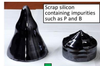
Melting of Si by electron beam (Evaporation of impurities)
